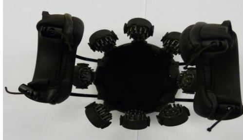
Figure 23. Inside view of DSI-7 showing areas that contact skin.
