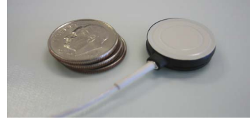
Fig. 1 QUASAR capacitive biosensor with 10c coins for scale.
