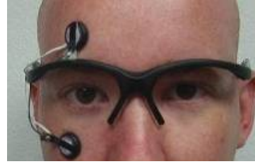
Fig. 10. Glasses with integrated QUASAR biosensors for measurement of EOG.
