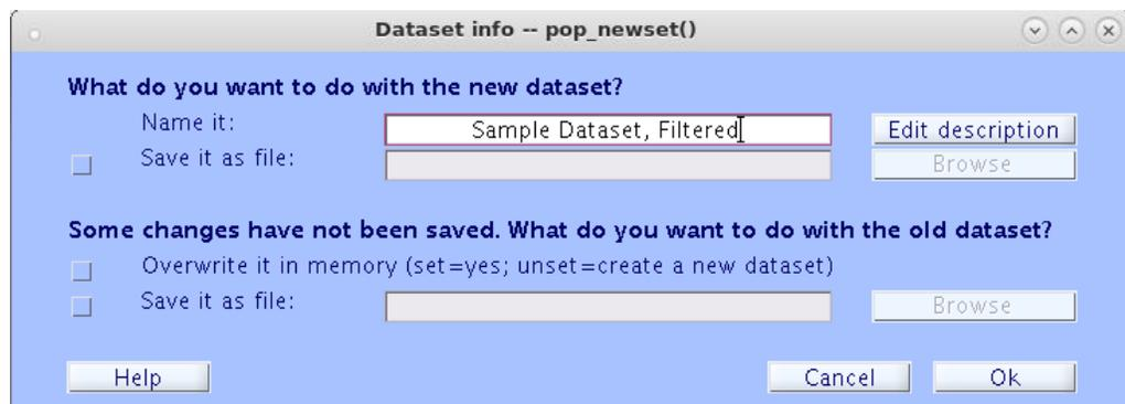
In this window, by default, if you hit “OK”, it will put the filtered data into a new dataset in EEGLAB. You may label the new dataset here by altering the name in the first dialogue box. As an example, the label has been changed from “Sample Dataset” to “Sample Dataset, Filtered” manually in order to differentiate the former dataset from the new one.
